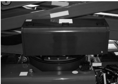
Fig. 119 Aerial part distributor protection
