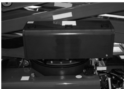
Fig. 107 Aerial part distributor protection
