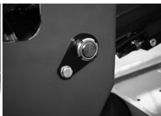
Fig. 23 Bolts to stop rotation
